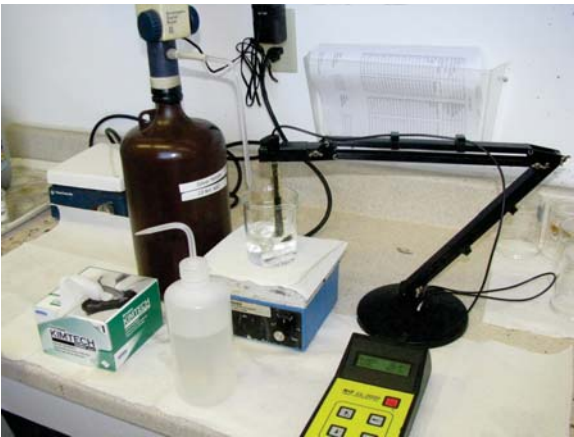
A lab titration process quantifies the chloride content in concrete and grout. (Photo courtesy of SCS)
