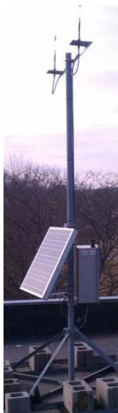
40 DCUs receive radio signals from 40,000 MTUs and send data via cell phone to Utility Billing System Database
