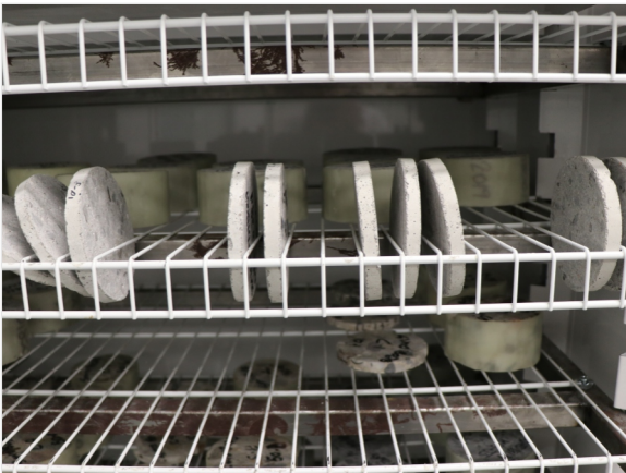
These concrete samples were cut into slices to reflect different depths from the concrete surface. They are ready to be tested for chloride-ion and moisture content. (Photo courtesy of VSL)
