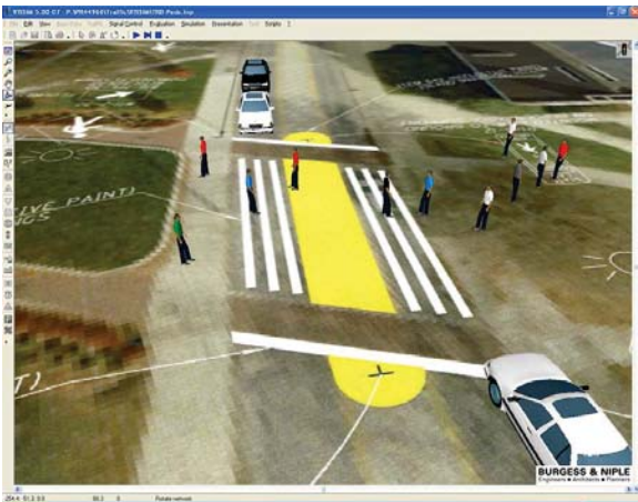
Figure 7 – Screenshots for Existing and Proposed Pedestrian Crossing Simulation
